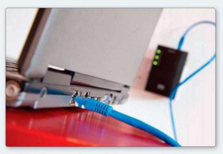
As before, connect one end of an ethernet cable to the powerline adaptor, and the other to your laptop, desktop, media player or games console. Now turn on the adaptor. That's most of the physical work done.
