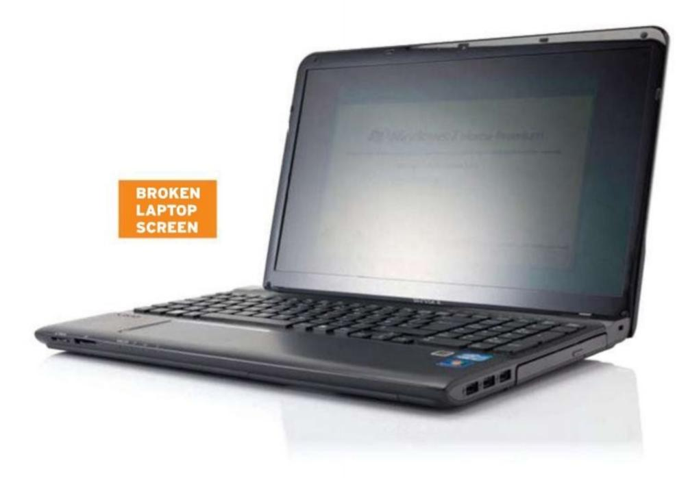
First, check the extent of the damage to the screen. It could be that the backlight has broken, but some or all of the screen pixels may still be intact. Try shining a light on the screen to see whether you can make out a faint image of the Windows desktop on the black screen. If you can, you may be able to see enough to be able to enable the external display using the Windows Mobility Center. Search for it from the Start menu (or press Windows, X), then look for External Display.
