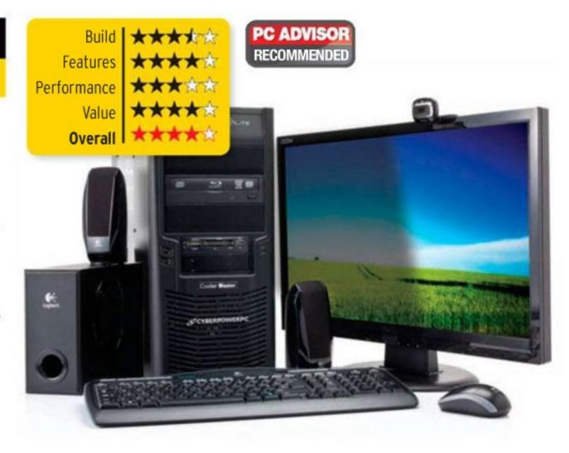
Like most family PCs, the Ultra Scylla SE has a 1TB hard drive, but no SSD. Wi-Fi support is provided by a small card plugged into the motherboard, which is neater than Chillblast's USB solution and allows for a decent-size antenna to be fitted.
