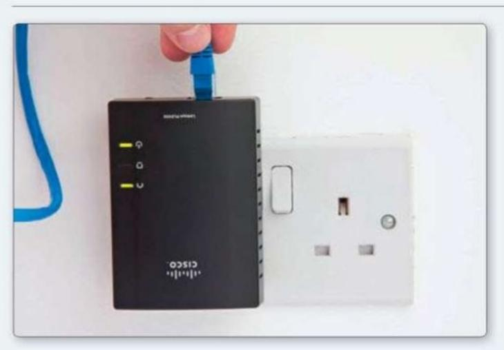
On the assumption that you have two matching powerline adaptors, plug one into a mains socket and turn it on. Avoid plugging the adaptor into an extension lead or surge protector, since these can interfere with its signal.
