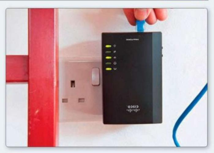
Plug your second powerline adaptor into a mains socket in the room into which you want to extend your home network. Remember to place the adaptor in a socket close to your computer or networking device.
