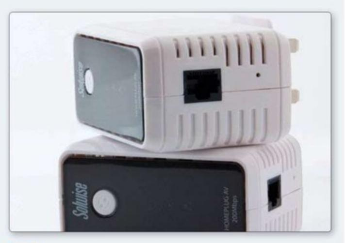
It's relatively easy to add another adaptor, even one from a different manufacturer. We connected a Solwise 200Mbps device to our laptop via ethernet, then pressed the button on the device. Seconds later it was connected to our network.
