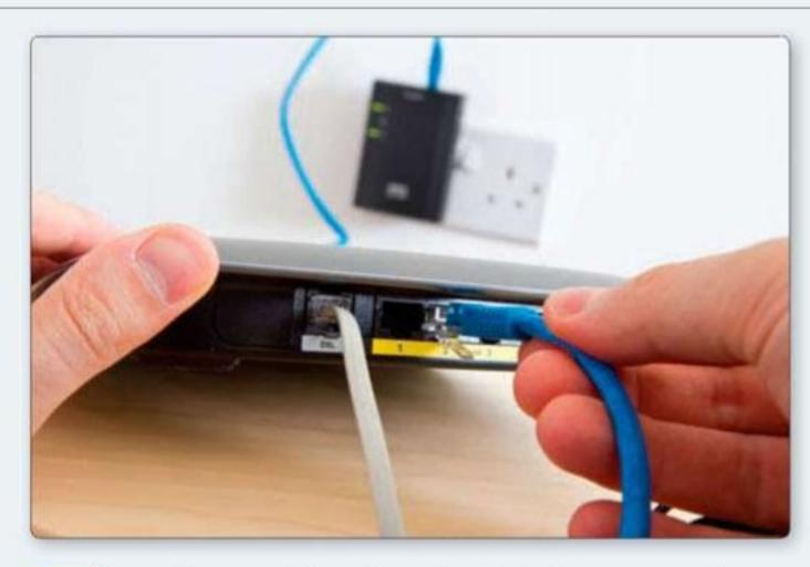
Connect one end of an ethernet cable to the corresponding socket on the adaptor, and the other end to your router. If it isn't obvious which port you should use, these are usually marked in yellow and carry a symbol comprising three squares joined by lines.
